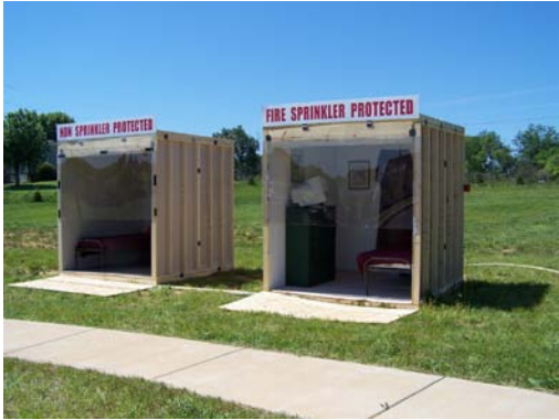
Side by side burn demonstration cubicles
